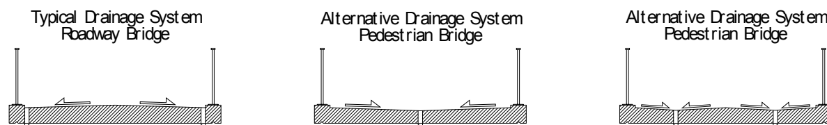
Fig. 6.7 Possible drainage schemes
