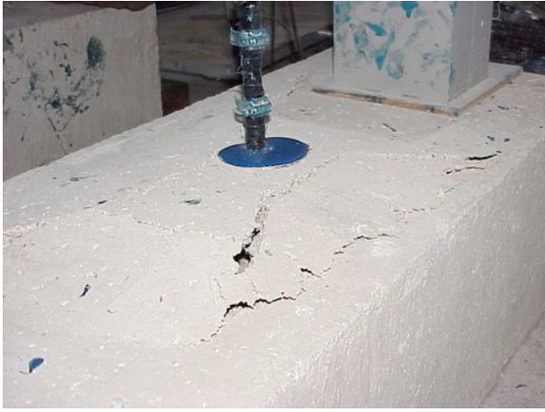
Fig. 13: Pullout failure of CFRP anchor
