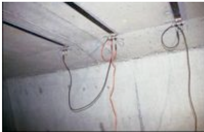
Fig. 8: Fast curing using heating device: (a) Schematic, (b) Photograph of end brackets.
