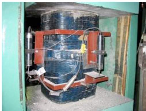
Fig. 12: FRP confined specimens after testing under axial stresses
