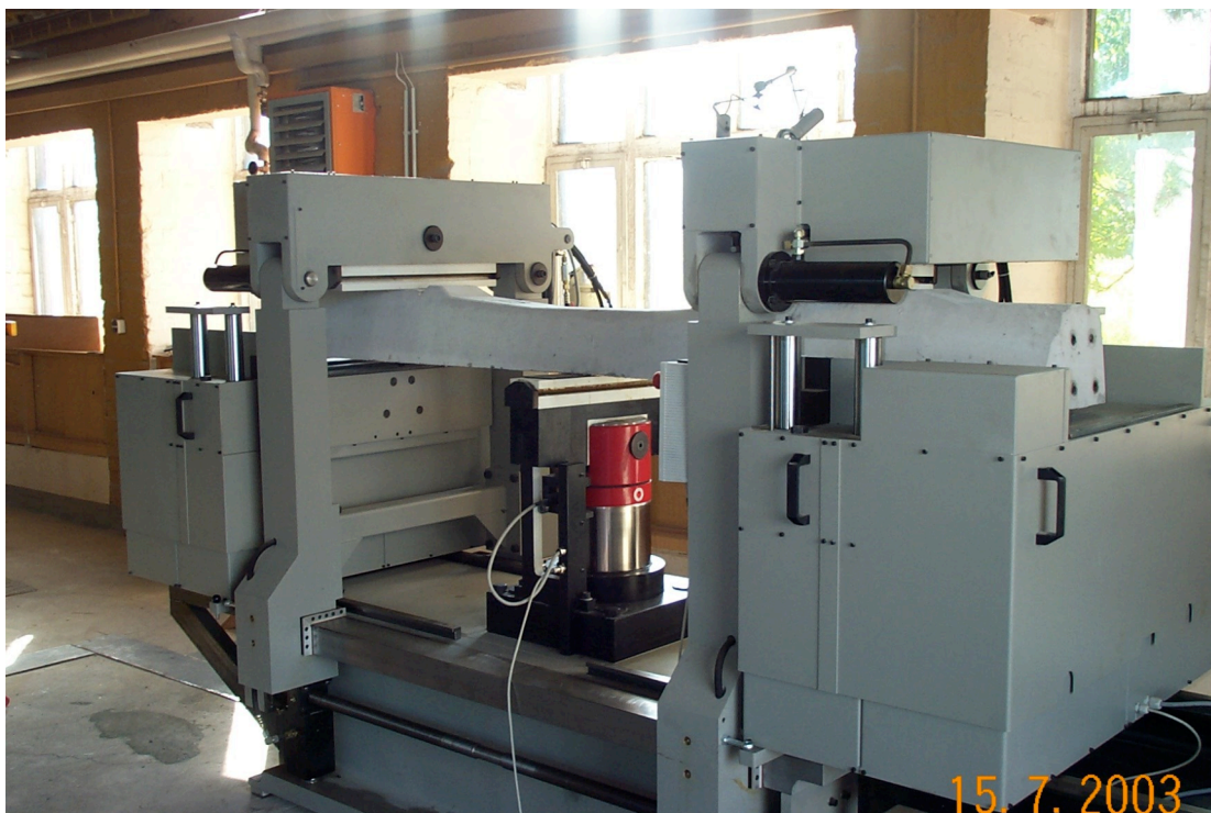
Figure 3-1: Dynamic testing of sleeper
