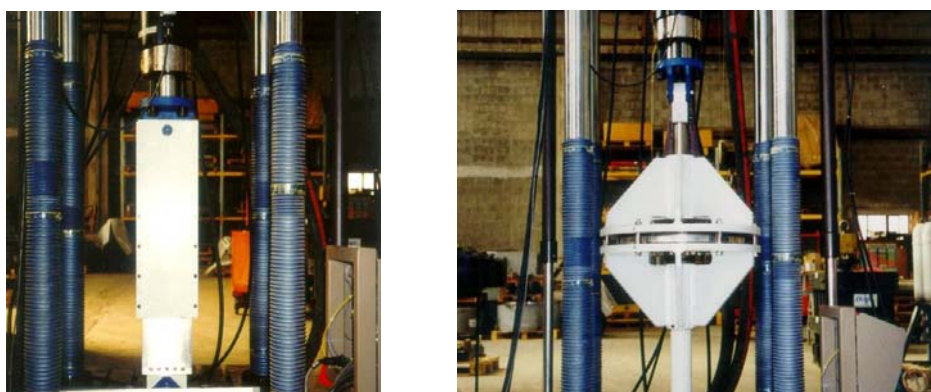
Fig. 6- 34: ER Dampers: linear (left) and rotating (right) working schemes (Marioni, 2002). (Figure available electronically on fib website; see production note on p. ii)
