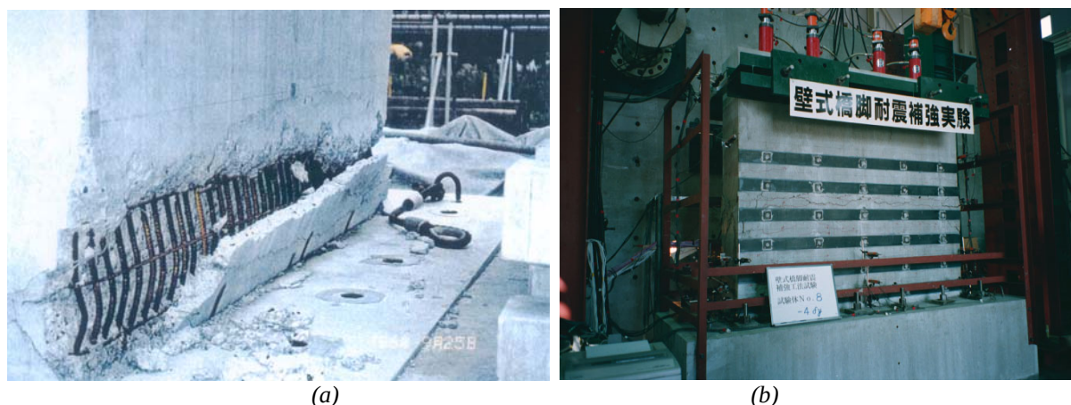
Fig. 11-20: Cyclic loading test on the retrofit of wall pier by steel jacket covered by reinforced concrete jacket with cross aramid fiber reinforced plastics rods: (a) As-built pier, and (b) Pier retrofitted using cross aramid fiber reinforced plastics rods [Tamaoki et al. (1996)] (Figure available electronically on fib website; see production note on p. ii)
