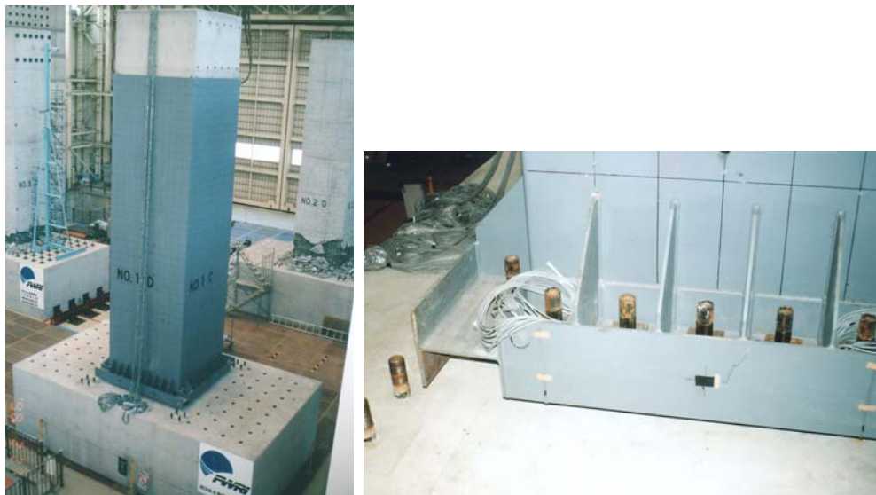
Fig. 11-9: Test models (9m tall and 2.5m x 2.5m section) for steel jacketing with controlled enhancement of flexural capacity (Figure available electronically on fib website; see production note on p. ii)
