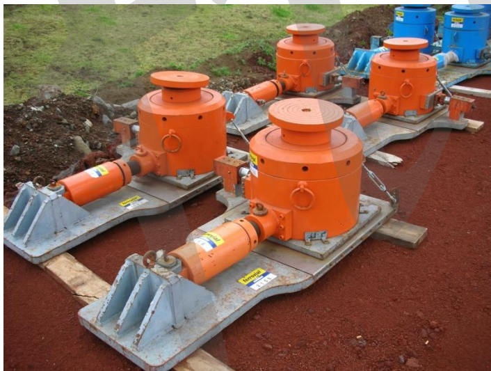
Figure 5-81: Hydraulic jacks to be used on the geometric adjustment operations
